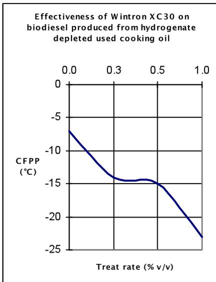
Cold filter plugging point (CFPP) – lowest temperature at which sample can pass through a filter<sup>2</sup>
